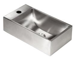
Overall dimension in mm Depth in mm Bowl dim. in mm Material Material thickness in mm Installation height in mm Gross weight in kg Net weight in kg Weight, pallet Pcs per pallet 400 x 230 x 111 100 318,5 x 208 x 100mm AISI304 1,2 900 3.78 2.64 272.00 72
