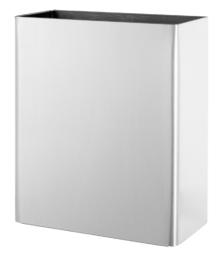
Overall dimension in mm Volume in L Material Material thickness in mm Installation height in mm Gross weight in kg Net weight in kg 356 x 432 x 165 26 AISI 304 0,8 559 (to bottom ) 3.90 3.50
