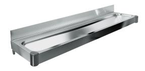
Overall dimension in mm 1800 x 430 x 140 Waste hole dim. in mm 52 Waste hole placement С Material **AISI 304** Material thickness in mm 0,9 Installation height in mm 850 Product load in N 1000 Gross weight in kg 13.10 Weight, pallet 116.70 Pcs per pallet
