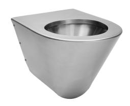
Overall dimension in mm Inlet dimension in mm Outlet dimension in mm Material Installation height in mm Product load in N 360 x 535 x 362 56,3 100 AISI 304 400 4000
