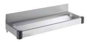
Overall dimension in mm 1200 x 430 x 140 Bowl dim. in mm 1130 x 300 x140 Waste hole placement С Material **AISI 304** Material thickness in mm 0,9 Installation height in mm 850 1000 Product load in N Gross weight in kg 9.60 Weight, pallet 140.20 Pcs per pallet 12
