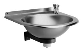
Overall dimension in mm Depth in mm Material Material thickness in mm Installation height in mm Gross weight in kg Made in 331 x 350 x 150 106 AISI 304 0,8 900/ 700/ 500 1.80 Norway
