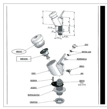
Apply some grease around the piston before assembly. If the O ringJR1 is damaged, the entire drink nozzle should be replaced.
