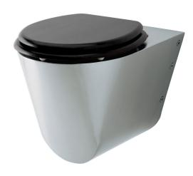
Overall dimension in mm 360 x 700 x 360 Inlet dimension in mm 56,3 Outlet dimension in mm 100 Material AISI304 Installation height in mm 400 4000 Product load in N Gross weight in kg 14.00 Pcs per pallet 15
