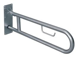
Overall dimension in mm Radius Material Material thickness in mm Installation height in mm Gross weight in kg Weight, pallet Pcs per pallet Ø32 / 800 x 100 x 303 32mm AISI 304 1,3 / 3 750 / 800 3.70 195.00 40
