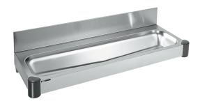
Overall dimension in mm 1200 x 430 x 140 Bowl dim. in mm 1130 x 300 x140 **Material AISI 304** Material thickness in mm 0,9 Installation height in mm 850 Product load in N 1000 Gross weight in kg 9.60 Weight, pallet 140.20 Pcs per pallet 12
